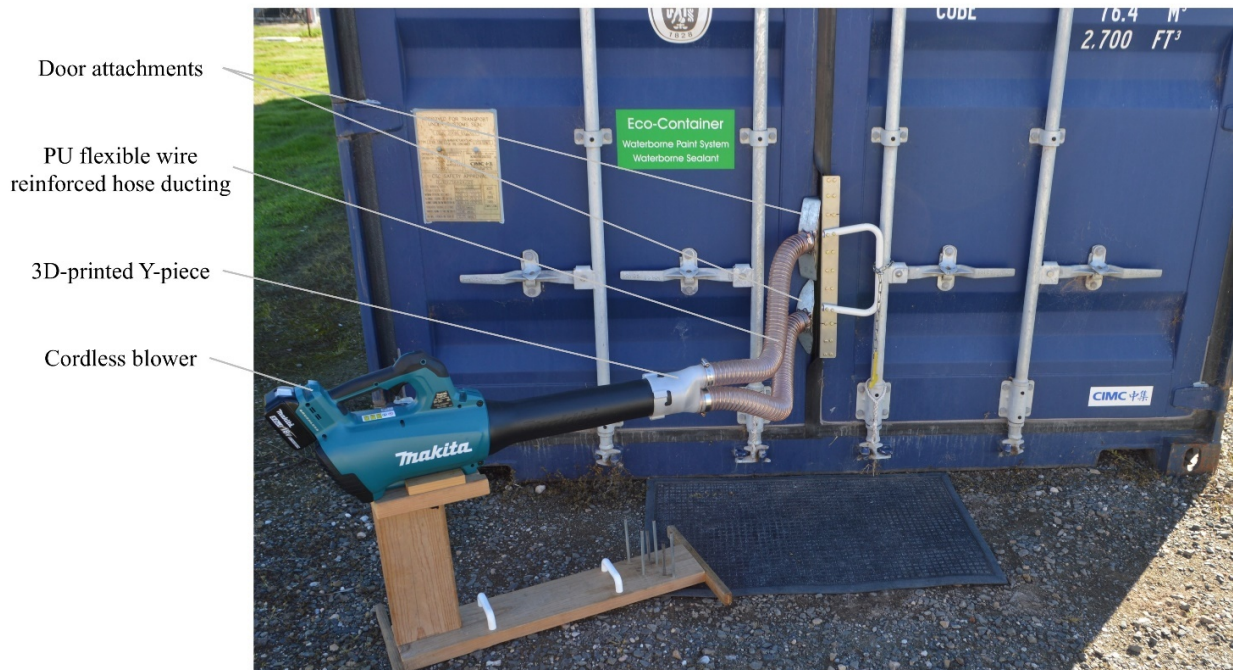
Figure 2. Cordless blower and adaptors for the passage of forced air into the container. The wooden support was a temporary addition for the purposes of this study.
